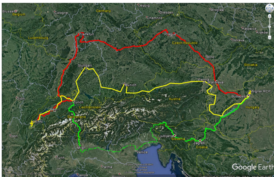
CERN's data centres in Switzerland and Hungary are connected by three independent 100 Gb/s optical fibre cables.
